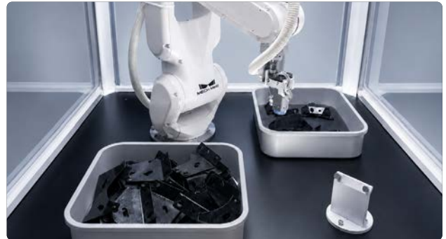
High-Precision Loading of Ultra-Thin Reflective Sheet Metal Parts
