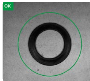
O-Ring Diameter Inspection
