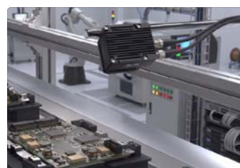
Semiconductor Component Presence & Orientation Inspection
